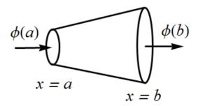
Figure 1: This is a schematic of the rod with variable cross-sectional area that the thermal energy flows through (integral formulation).
